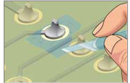
Figure 1 Scrape away damaged or unwanted coating.
