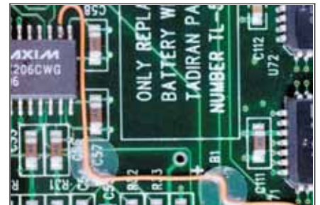
Figure 4 Bond wires using tape dots or strips.
