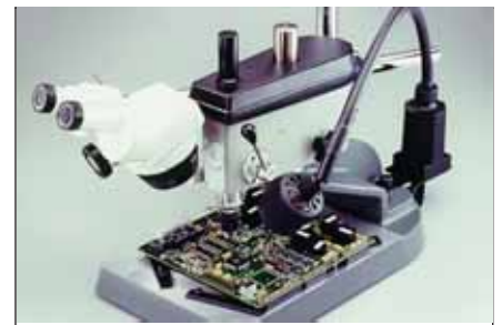
Figure 2 Precision drill press with microscope attachment.
