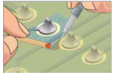
Figure 2 Apply hot air to the work area and remove overcured coating.
