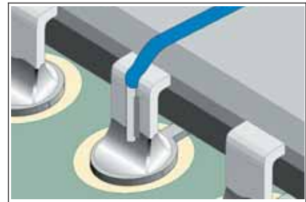
Figure 15 Not Recommended Wire soldered to lead, wire over component.
