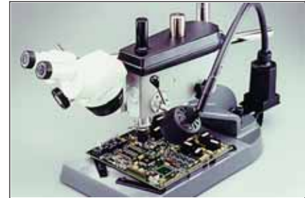
Figure 5 Precision Drill System used for milling the Teflon sleeved hole.
