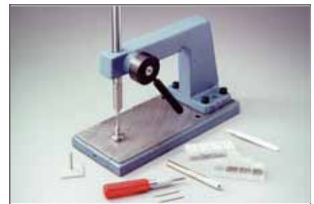
Figure 2 Set the eyelet using an eyelet press.
