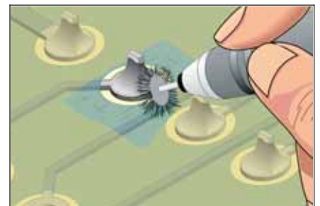
Figure 3 Rotary brushes are best used to remove soft coating.
