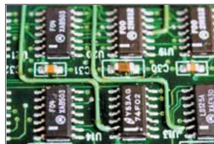
Figure 6 Adhesive coated wires are heat bonded.
