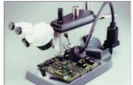
Figure 1 Drill press shown with PC board pinned in place.
