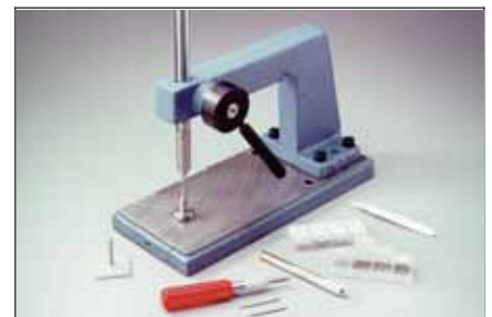
Figure 3 Set the eyelet using an eyelet press.
