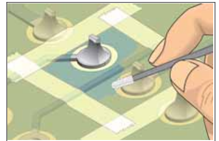
Figure 2 Apply solvent with foam swab to remove coating.
