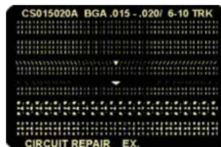
Figure 2 Select a replacement pad that matches the missing pad.
