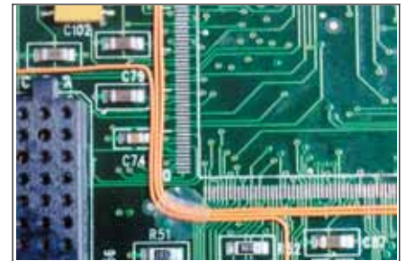
Figure 1 Route jumper wires.
