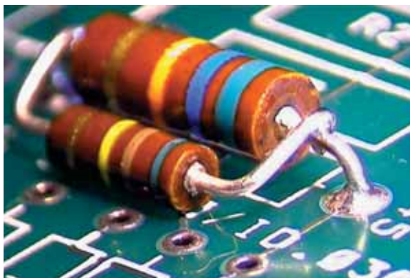
Figure 3 Axial lead component soldered to adjacent axial lead component. Note: Added component may be stacked vertically or horizontally.
