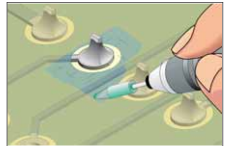
Figure 2 Rubberized abrasives used to remove thin, hard coating.
