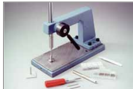
Figure 5 Set the eyelet using an eyelet press.
