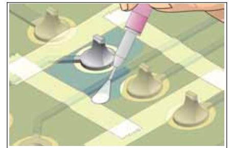
Figure 2 Remove coating using micro blasting system.
